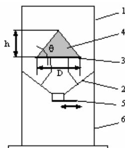
Fig. 2 – The device for determining the drained angle of repose.
