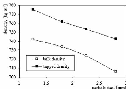
Fig. 5 – Effect of urea particle size on bulk and tapped density.
