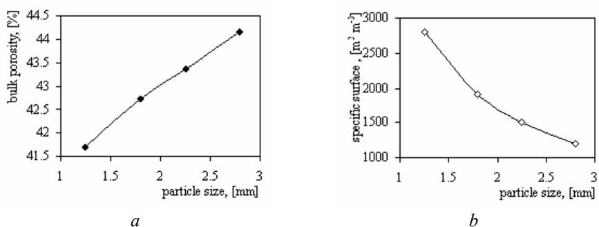
Fig. 6 – Effect of urea particle size on bed porosity (a) and specific surface area (b).
