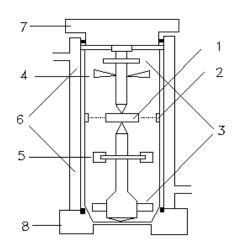
Fig. 6 - Gas - liquid reactor used by Siminiceanu (2005)
