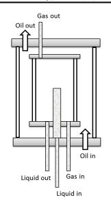
Fig. 1 – Gas–liquid contactor used by Cullinane and Rochelle.
