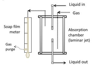
Fig. 2 – The laminar jet apparatus used by Aboudheir (2003).
