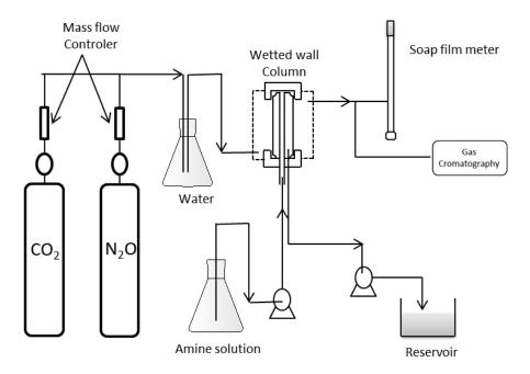
Fig. 3 – The schematic experimental equipment used by Yoon (2003).
