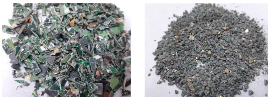
Fig. 2 – PCB sample after coarse and fine grinding.
