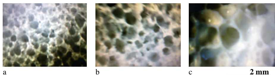
Fig. 2 – Appearance of the geopolymer foam specimens a – variant 1; b – variant 2; c – variant 3.
