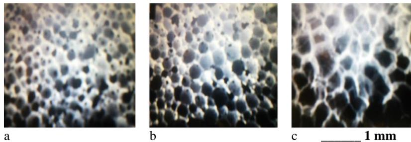
Fig. 3 – Microstructural appearance of foam glass gravel specimens
