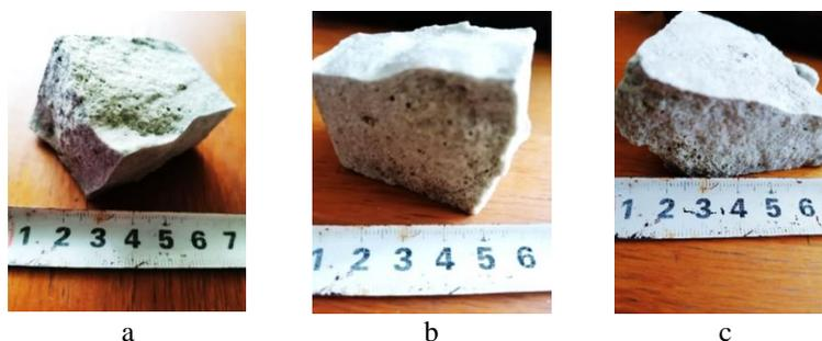
Fig. 2 – Aspect of foam glass gravel lumps
