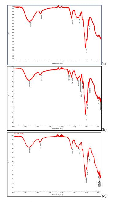
Fig. 1 – FT-IR spectra of (a) hardwood xylan (Xy); (b) acetylated xylan (XyAc); (c) AKD hydrophobized xylan (XyAKD).
