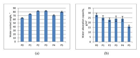
Fig. 3 – The water barrier properties of xylan coated papers.
