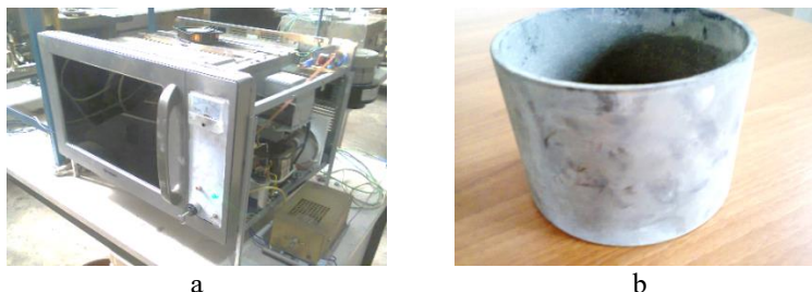
Fig. 1 – Experimental microwave equipment. a – 800 W-microwave oven; b – protective ceramic tube.
